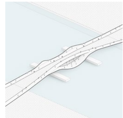
Floating supporting structure that allows the bridge to adapt to the water level.
